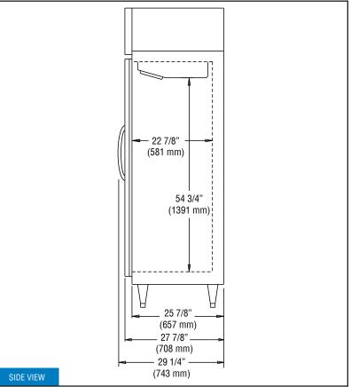
**IMPORTANT NOTE:** If the cabinet is located directly against a wall and/or under a low ceiling, a <u>minimum</u> clearance of 12" is required on top and 3" on sides and rear.
